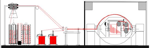
CORDE FLESSIBILI DA 1.5 A 35 mm² FLEXIBLE STRANDS FROM 1.5 TO 35 mm<sup>2</sup> CORDE REGOLARI DA 2.5 A 25 mm² REGULAR STRANDS FROM 2.5 TO 25 mm<sup>2</sup> RIUNIONE DI CAVI ISOLATI IN P.V.C. fino A 12 mm CABLES UP-TO DIA. 12 mm. Insulated in P.V.C.
